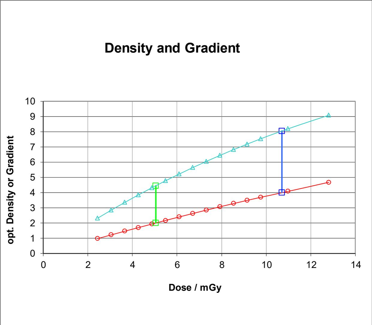
**Figure 1:** Mean optical density  $\langle D-D_0 \rangle$  (red curve) and mean gradient  $\langle G \rangle$  (blue curve) of eight films as function of exposure dose  $K$ .
