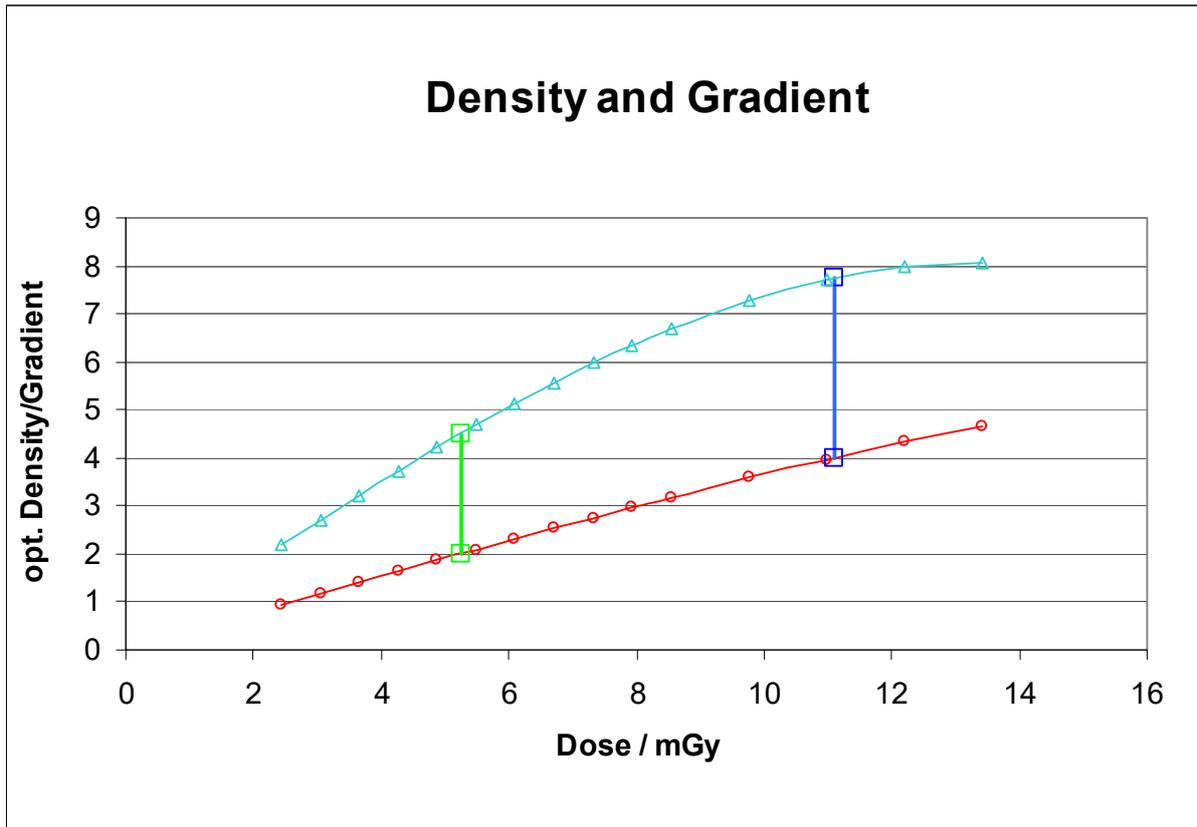
**Figure 1:** Mean optical density  $\langle D-D_0 \rangle$  (red curve) and mean gradient  $\langle G \rangle$  (blue curve) of eight films as function of exposure dose  $K$  (Reg. No. BAM 17-20).
