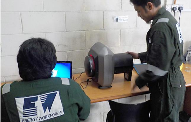
The CR 35 NDT is Energy Workforce's first foray into digital radiography. Previously, only conventional film was used for radiographic inspection and according to Mr. Quayum, Radiation Protection Officer: "Compared to film, the quality is much more reliable. Imaging plates are also easier to handle and the processing time is a lot faster".
