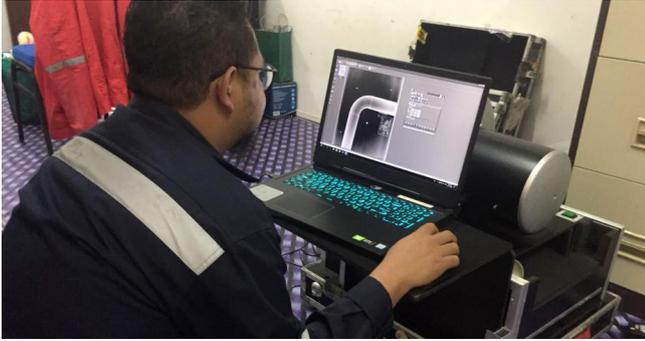
Danamin has been using the HD-CR 35 NDT system for pipe profile inspection since 2007 and initially acquired the system to fulfill an inspection requirement from Petronas Chemicals MTBE in Kuantan. Other customers taking advantage of Danamin's computed radiography capability include BASF Petronas in Kuantan and Idemitsu Petrochemical in Johor.
