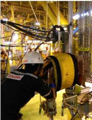
The typical inspection workflow for Danamin is to expose the imaging plates on-site and then bring them back to headquarters for scanning, or if the location is far away, the radiographic team will scan the imaging plates at a temporary base. Both scanning and image evaluation is performed by a single fully-trained operator.
