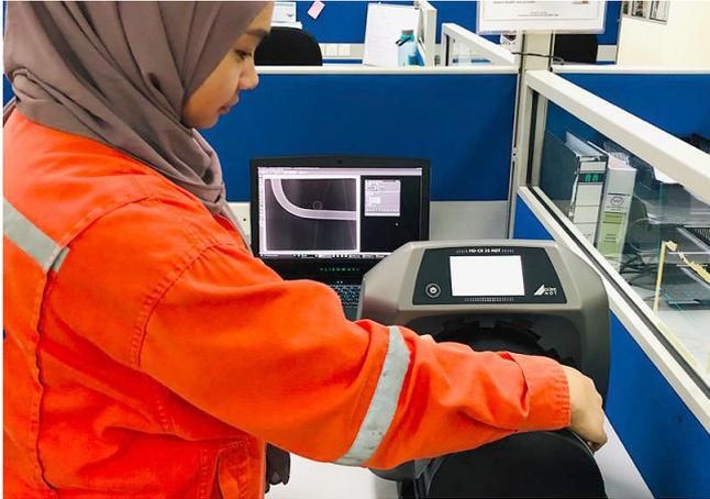
Winner Inspection has been a user of DÜRR NDT's HD-CR 35 CR scanner since 2017 and utilizes it primarily for pipe wall thickness profiling during service and production stop using Iridium-192. The HD-CR 35 system is also used to inspect weldment, flange and valve conditions in oil and gas plants and platforms.
