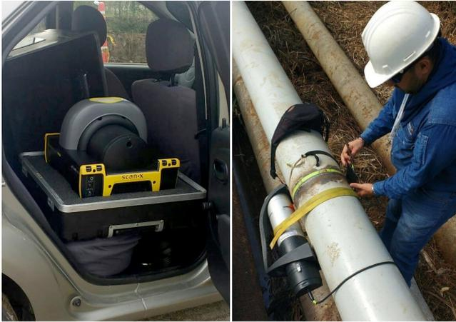
The company specializes in radiographic testing of welds. "Our main tasks are field inspections of welds on in-use pipelines with diameters that variate from 2 to 6 inches" commented Omar Garza.
