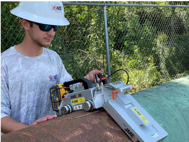
With a rapid magnetic deployment system, the DXB:1 can be positioned by a single person in less than a minute. The system is attached using permanent magnets, meaning in the event of a loss of power the unit will remain firmly attached to the pipe. Combined with an X-ray or gamma source, the system is fully integrated with crawler operations and produces the full weld on one single image with one shot.
