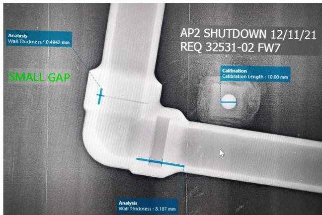
Stork Technical Services has been using the CR 35 NDT Computed Radiography scanner since 2019 and uses it with Iridium-192 in combination with high-sensitivity white imaging plates to perform Corrosion-Under-Insulation (CUI) radiography and digital gap shots which are used to check for gaps in socket welds. The scanner sees heavy use of up to 60 hours per week and has been used to acquire more than 5000 X-ray images to-date.
