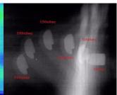
Imaging Example: The images above show a sequence of six exposures, taken 50µsec apart, on a single CR plate, of a 30-06 bullet (moving right to left) striking a bullet proof (Kevlar) vest. The exposures were created using 150kV pulsers. Each x-ray pulse lasted 70nsec.
