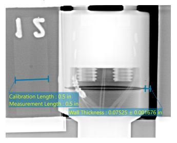
As it can be seen in the image above, the user can just zoom into a region of interest using the zoom magnifying function in the D-Tect X software. Then, they can then use either the wall thickness measurement tool or the line measurement tool to precisely measure the amount of joint penetration.
