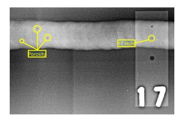
One example of how digital imaging has helped them with the evaluation process can be seen in the image above. In the past, while using film, the 1T hole in the IQI along with the three small pores in the groove weld may not have been detected. Now, however, they can increase the probability of detection by using digital imaging filters built into the D-Tect X software along with adjusting the brightness and contrast.
